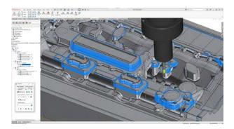
SolidCAM High-Speed Machining (HSM) offers unique machining and linking strategies for 3D high-speed toolpaths. It smooths the paths of both cutting moves and retracts, wherever possible, to maintain a continuous machine tool motion – an essential requirement for maintaining higher feed rates and eliminating dwelling.
